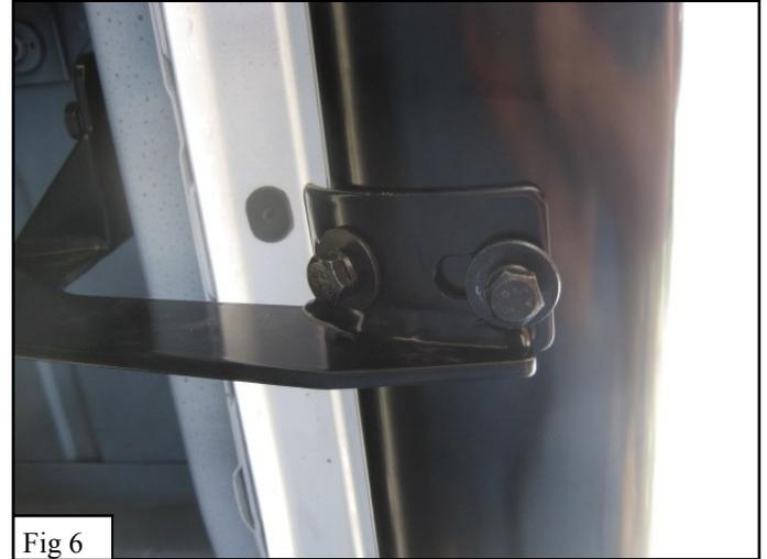
11. Level and adjust step bar as needed then fully tighten all hardware to the following specifications: 1/2" hardware to 60ft-lbs, M12 hardware to 40-45 ft lbs, M10 hardware to 30-35 ft lbs, and M8 hardware to 25-30 ft lbs.
