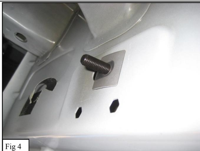
7. Move to the rear drivers side and locate the tape covering the oval hole in the body. Repeat **Step 6** to install the rear mounting bracket (9).
