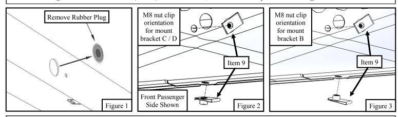
3. Take the mounting brackets and install the bracket and associated hardware loosely to it's corresponding positions see **Figures 4, 5, 6, and 7.** Brackets used for passenger side are (1) bracket C (Item 4) and (1) bracket D (Item 5). The driver side will use the remaining (2) bracket B (Item 3). Do not fully tighten hardware at this time. **Note:** Bracket location is critical.
