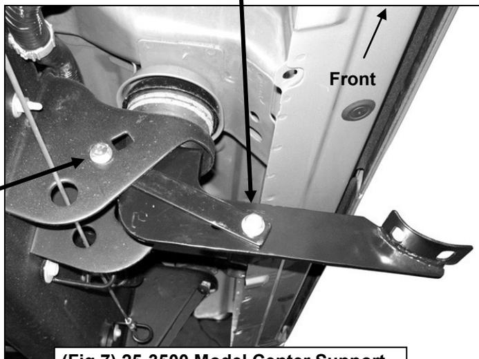
**(Fig 7) 25-3500 Model Center Support Bracket Installation Pictured.**
