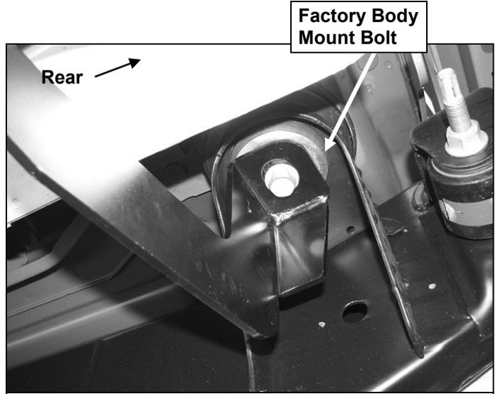
**(Fig 2) Driver side rear mounting bracket pictured**
