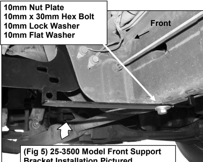
**(Fig 5) 25-3500 Model Front Support Bracket Installation Pictured**
