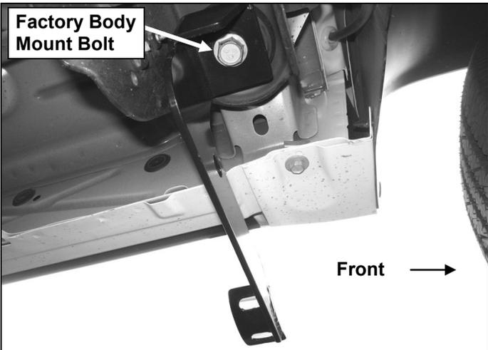
**(Fig 1) Driver side front mounting bracket pictured**
