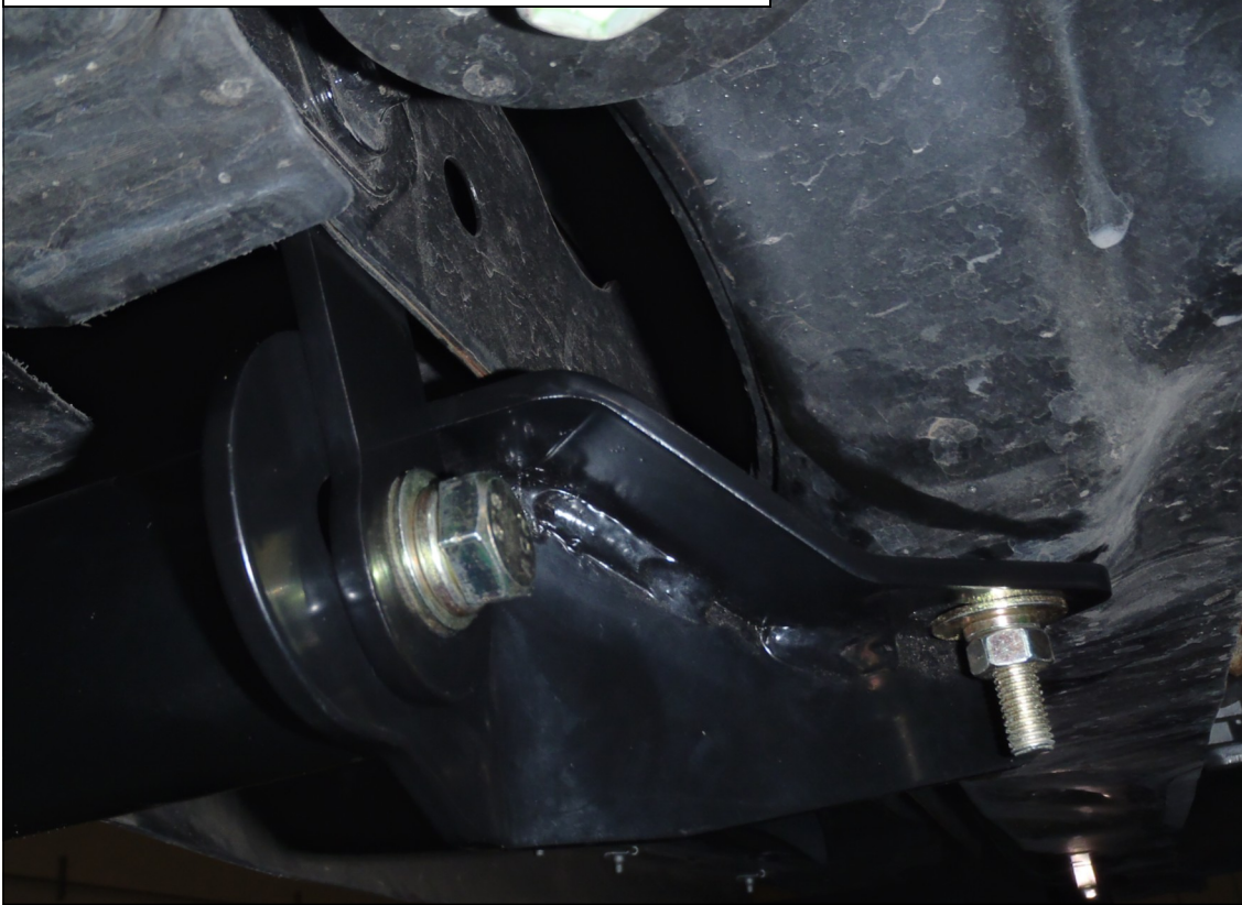
(Fig 5) Contour bar mounted to drivers side bracket
