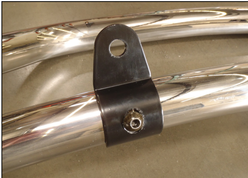
(Fig 8) Light tab installed on bar
