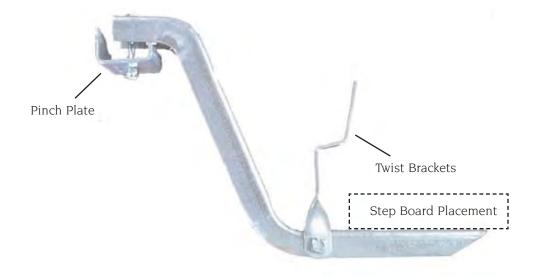
**STEP 3:** Attach the pinch plate portion of the brackets to the truck at the Cab Rail and tighten the 5/16" x 2½" Hex Head Bolts and 5/16" Nylocks. Note: All the Brackets should be loosely hanging from the truck.
