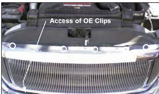
FIGURE 1 - OE Grille Shell removal
