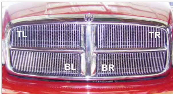
FIGURE 1 - Correct Placement of Grille Inserts
