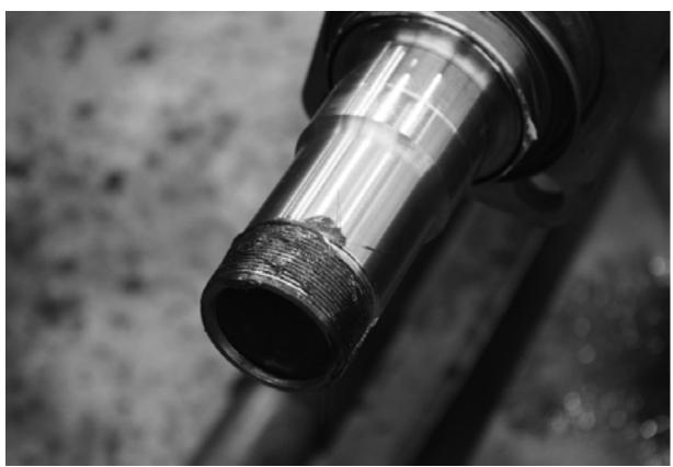
Apply a liberal amount of bearing grease to the spindle threads.
