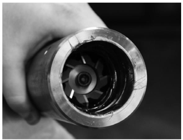
Slide the cutting head/boring shaft into the boring tool housing.
