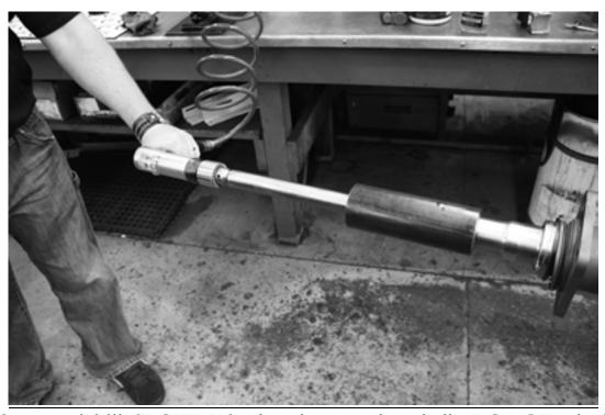
Using a low speed drill, <u>SLOWLY</u> begin to bore out the spindle. <u>DO NOT</u> spin the cutter too quickly or apply too much pressure. Keep the tool well lubricated during the cutting process. Once completed, repeat for the other side. After both sides have been successfully bored out, thoroughly clean the housing to remove all metal shavings.
