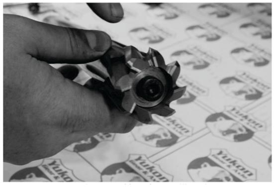
Begin by securing the cutting head and tightening down the bolt.
