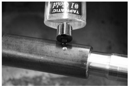
Apply a liberal amount of cutting fluid through the oiling port on the boring tool housing. You will need to add more fluid as you go. It is <u>VERY IMPORTANT</u> to add cutting fluid as necessary to make sure the cutting head has proper lubrication. FAILURE TO DO THIS WILL RESULT IN PERMANENT DAMAGE TO BOTH THE BORING TOOL AND YOUR HOUSING.
