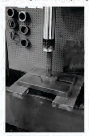
Use the press to gently push the axle down to safely and easily remove the bearing.
