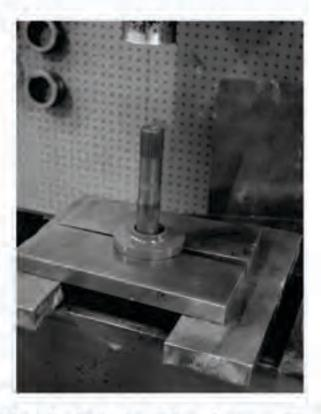
If using a press, place the axle puller body & axle into the press. The top lip of the puller body is supported by the press plates. Make sure you have enough room between the bottom of the axle and the floor for bearing removal before operating the press.
