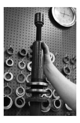
If using the axle bearing puller with a Yukon® carrier bearing puller, place the carrier bearing puller body over the top of the axle.
