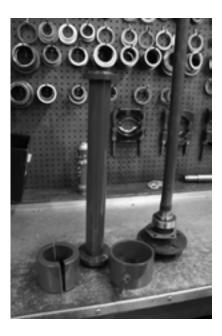
This axle bearing puller comes with one (1) set of clamshells, one (1) puller body, and one (1) clamshell retaining sleeve.
