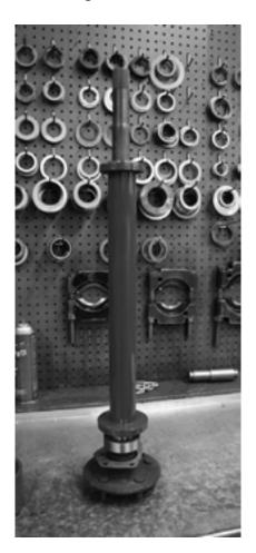
Begin by sliding the body of the puller over the axle shaft and seating it against the bearing.
