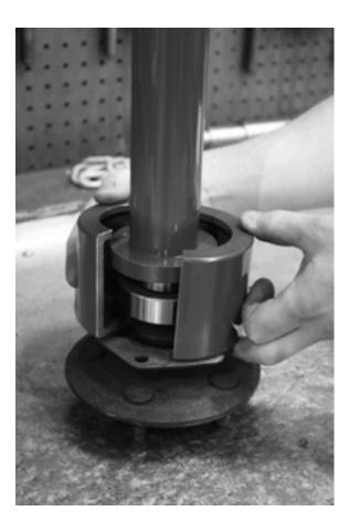
Place the clamshells on the puller and axle. The bottom of the clamshells goes under the axle bearing. The top of the clamshells should clear the lower lip of the puller.
