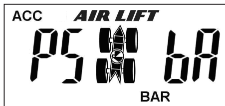
Setting the pressure units
