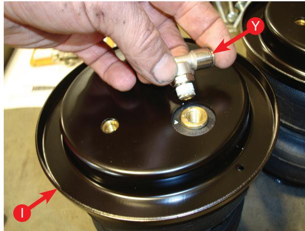
Set roll plate (I) over the bellows and install the fitting (Y) as stated. Repeat for both bellows.
