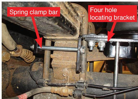
With the spring clamp bar tight so that the lower bracket is up against the stock U-bolts, the four hole locating bracket should be forward and behind the U-bolts as shown. Note the lower bracket being parallel with the leaf spring.
