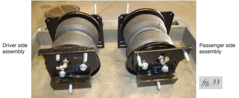
**ATTACHING THE ASSEMBLIES TO THE FRAME**
