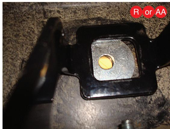
For the passenger side, before inserting the upper brace hardware, make sure that the 1/2" thick washer (R) or (AA) is installed in between the brace and frame (see Step 2). **Note:** The 1/2" thick washer (R) is not a half inch thick. It has a 1/2" hole and is a thick washer.
