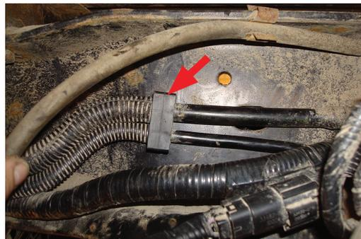
If equipped, this emissions/fuel line retaining clip must be pulled away from the frame in order to install the upper frame brace (D).
