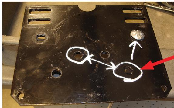
Passenger side bellows mounting holes shown in location to the 3/8"-16 x 10" carriage bolt previously installed. When installing on the bellows, make sure the bracket edge facing you is on the fitting side of the bellows.
