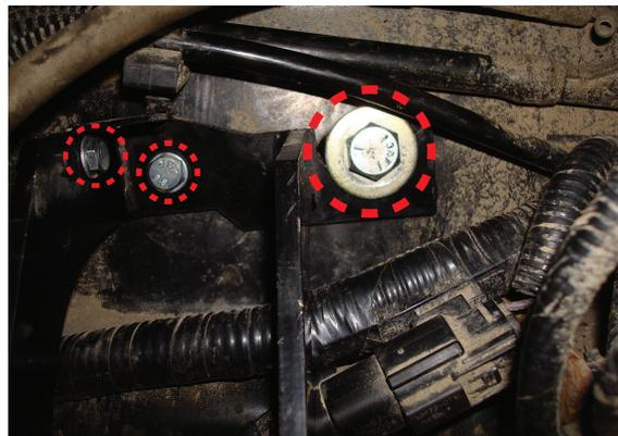
Driver side brace shown with supplied hardware in place. Existing 5th wheel hardware which may have been removed may look different.
