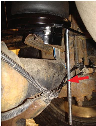
Make sure when setting the right side in place (passenger side) that the 3/8"-16 x 10" carriage bolt goes on the outside (backside) of the hard brake/ABS line.
