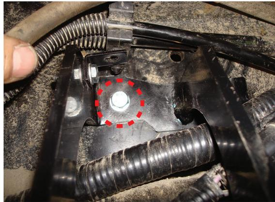
Attach the bracket to the frame using the M8 hardware noted.
