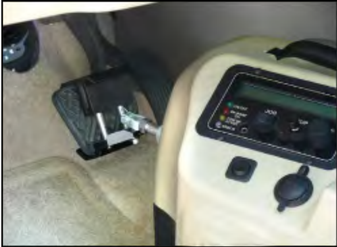
Fig. 1 Place claw on brake pedal
