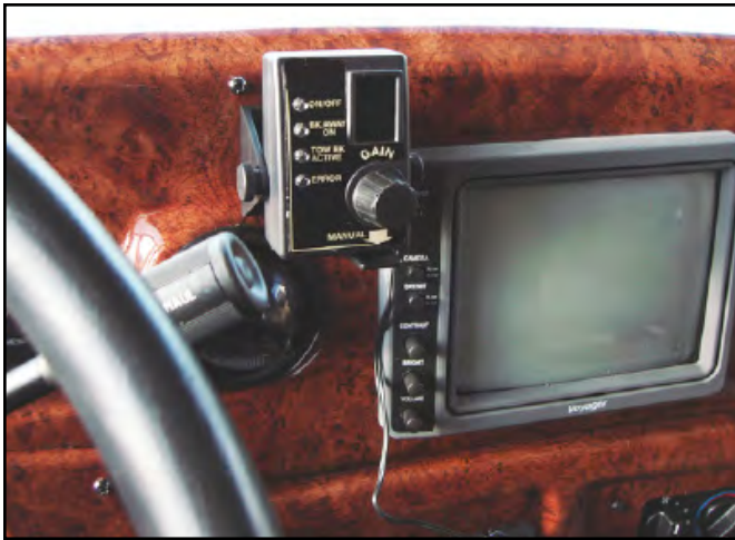
Fig. 5 RF in-coach controller mounted on dashboard
