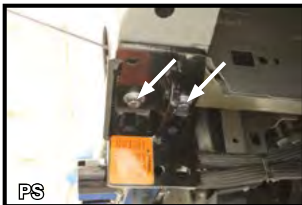
9. Attach baseplate to the underside of the bumper using the existing two (2) holes. Use a 3/8"-16 x 2" bolt, 3/8" flat & lock washer with a 3/8" nut plate for each hole.
