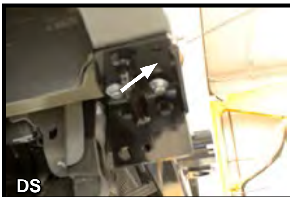
10. Using the endplate as a template, drill an additional hole using a 13/32" drill bit. Install a 3/8"-16 x 1-1/2" bolt, 3/8" lock washer and 3/8" nut plate into hole.
