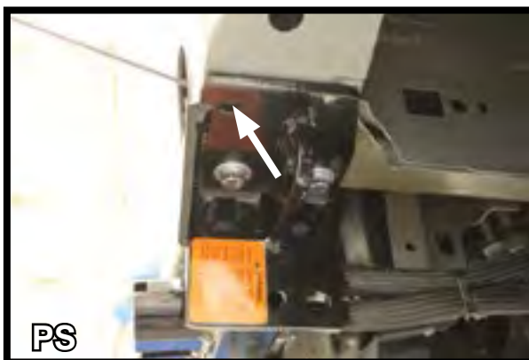
10. Using the endplate as a template, drill an additional hole using a 13/32" drill bit. Install a 3/8"-16 x 1-1/2" bolt, 3/8" lock washer and 3/8" nut plate into hole.
