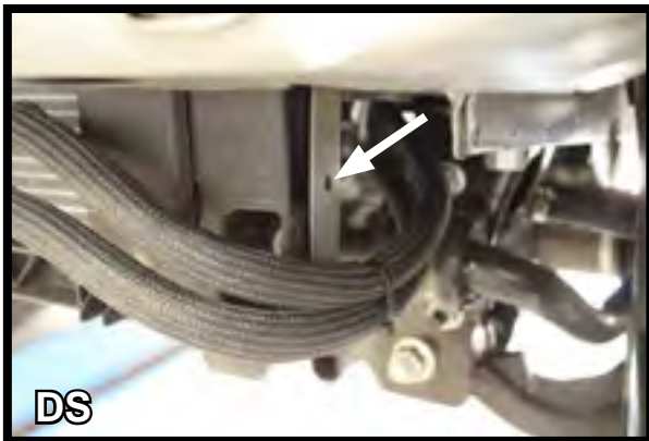
7. On the driver side only, move the coolant lines down and remove the push pin.
