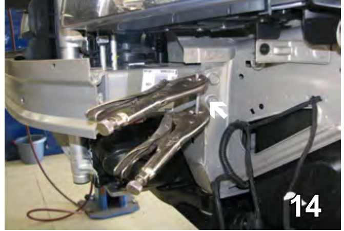
14. Using vice grips, bend the metal edge over and flatten with a hammer. Do this on both sides.
