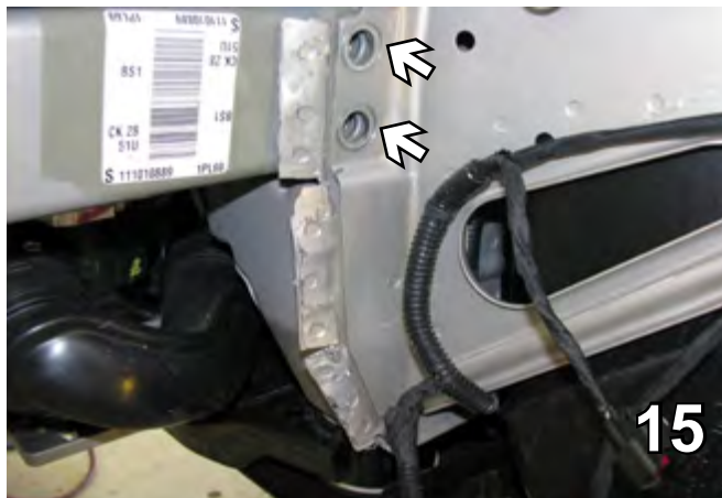
15. Using an 18MM socket and a wrench on the other side, remove the two metric bolts next to the flattened area. Do this on both sides. Set bolts aside to be reinstalled later.
