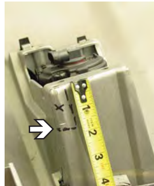
12. Using the utility knife, on the inside of the fascia trim the fog light housing bumps, on the bottom trim back 2" and on the top trim 1 1/2", flush with the plastic surface.
