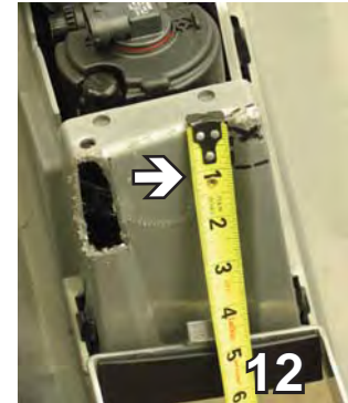
12. Using the utility knife, on the inside of the fascia trim the fog light housing bumps, on the bottom trim back 2" and on the top trim 1 1/2", flush with the plastic surface.
