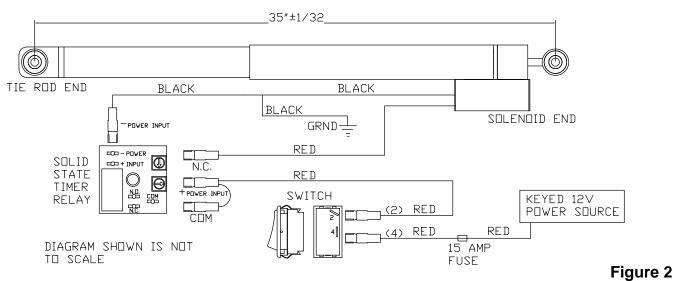
**A.** Route the two-wire harness from the TruCenter up to the motor home's front hood area. Locate a keyed 12-volt power source and a ground point.
