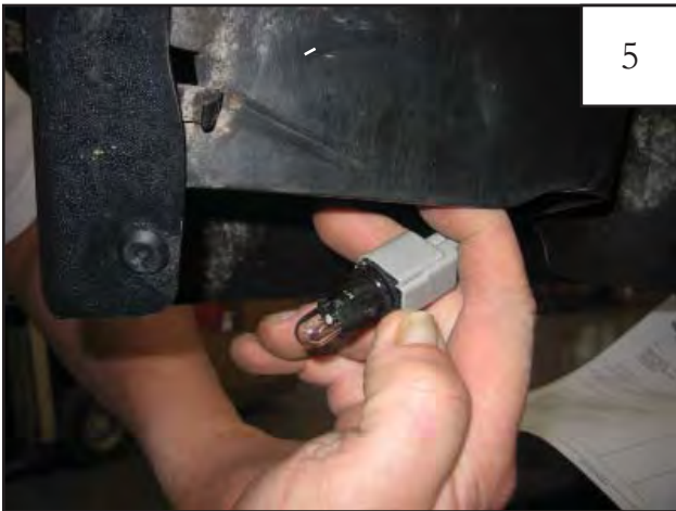
Once flare is free of fender, disconnect light connector. This will allow the flare to come away from fender completely. Remove light housing from factory flare; you will be reinstalling this later.
