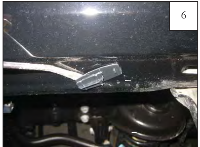
Using a pry tool or flat head screwdriver, remove any plastic clips that have remained in fender.
