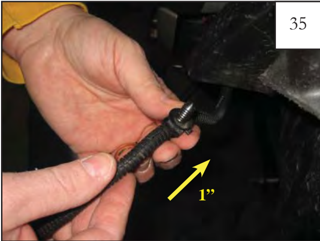
Slide the Christmas Tree Clip on light cord in towards vehicle body approximately 1"
