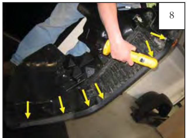
Use a drill with a 5/16" bit to drill through six plastic rivets along edge of flare/splash shield. Discard the flare, but retain the splash shield and inner structure.
