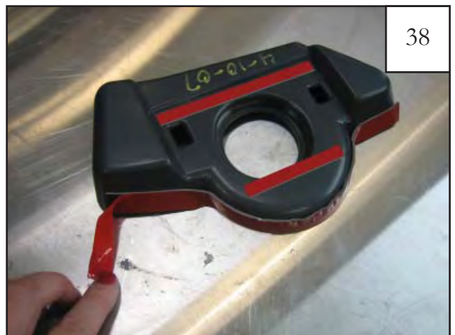
Peel liner completely from two pieces of 1/4" tape located on face of Light Pocket Inner Piece. Fold tape liner tab attached to long 1/2" tape upwards (do NOT peel liner from 1/2" tape in this step).
