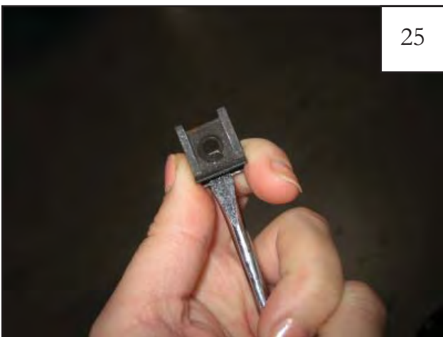
Use a flat head screwdriver to spread supplied #14 U-clips for ease fo installation.
