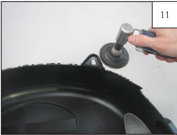
Sand mounting tabs flat using an angle grinder or sand paper.
