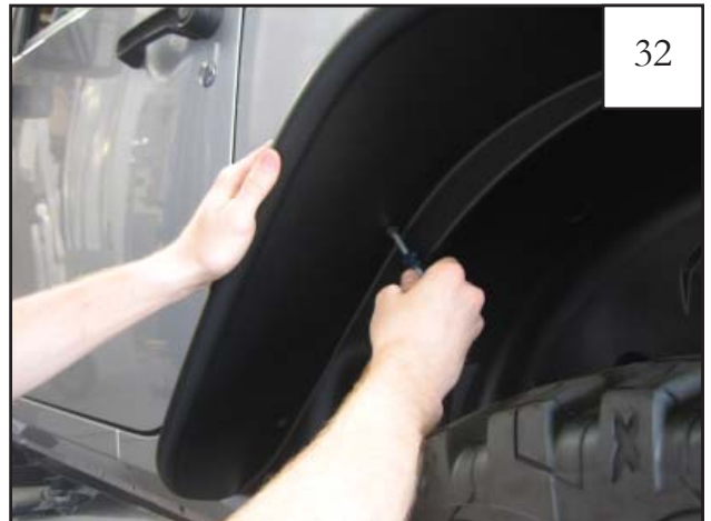
Hold flare in place on fender and start a pan head screw into each hole location and through the speed clip on inner structure (6 locations). Do not tighten.
