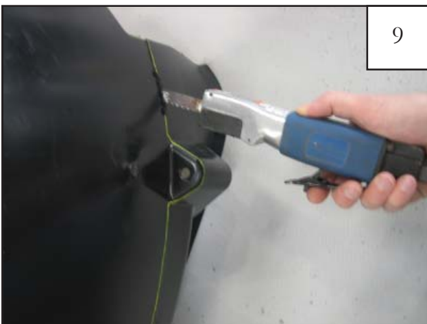
Using a metal hacksaw, pneumatic hand saw, or other suitable cutting device, trim the splash shield along the marked lines.
