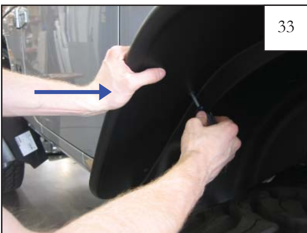
After all screws have been started, tighten the pan head screws by firmly pressing the flare toward the vehicle while tightening.
