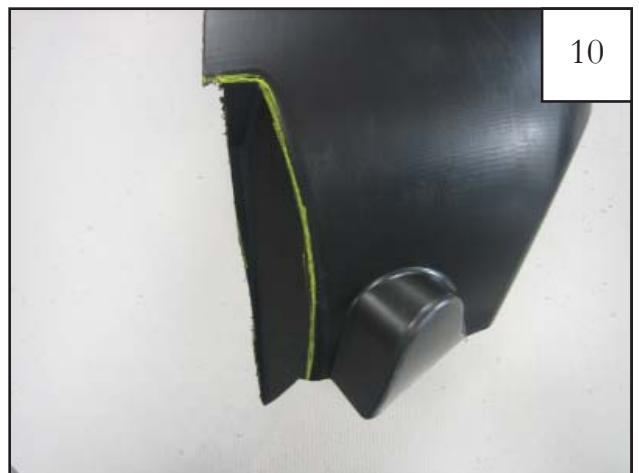
After trimming, mark the rear portion of the splash shield as shown and trim. NOTE: If trimmed too little, flare won't fit; if trimmed to much, shield won't stay behind flare.
