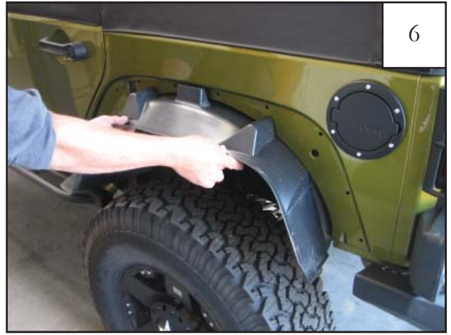
Hold the splash shield in place using supplied 1/4" Panel Retainers through factory holes halfway. Do not fully install Retainers, leave them half out. They are only used to hold splash shield in place for marking. See step 26 for locations.
