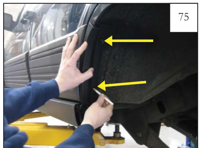
Hold cover piece over "dog leg" and mark inner wheel well through holes in part. If cover piece fits poorly more hammering is needed. Part is marked on the inside. Driver's side: LR5 for cover piece.
