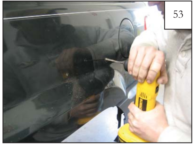
Drill holes in fender and bumper at marks with a 3/16" drill bit.
