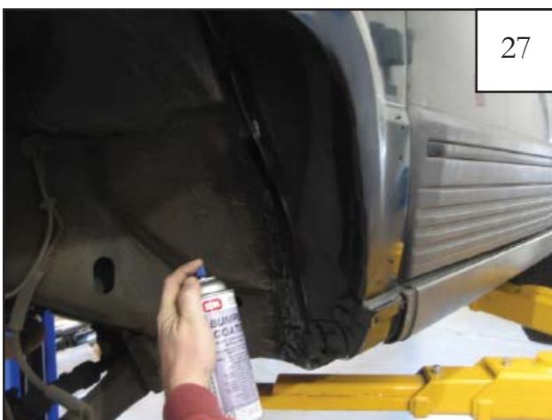
27 Using spray paint, repaint the sanded edge of the wheel well flange. NOTE: Be sure to cover the rest of the vehicle so paint does not get on other accessories such as side cladding.
