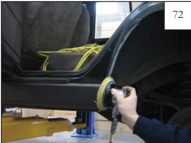
Open door. Sand the chipped paint along bent edge of the wheel well.
