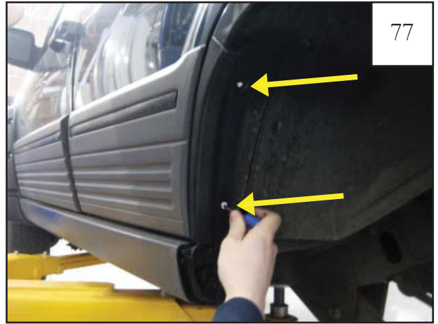
Place cover piece back on "dog leg" and fasten with two #8 pan head screws. Screws are white in picture for visibility.
