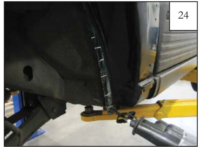
24 Cut along horizontal lines in pinch weld using reciprocating saw.
