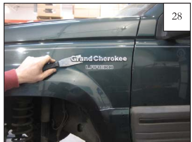
28 Using a putty knife, remove any decals. Buff residual adhesive off with adhesive remover disk.
