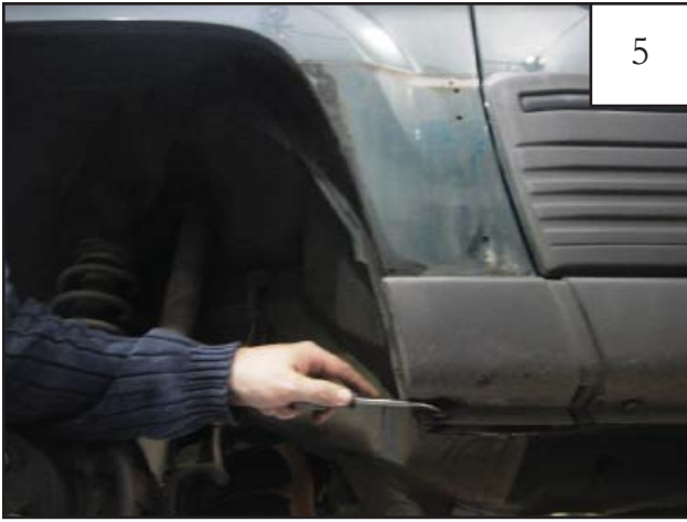
Remove one christmas tree fastener from bottom of lower side cladding.
