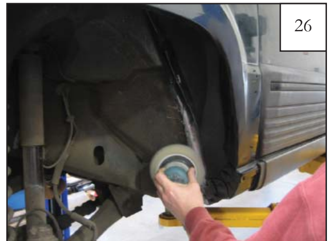
26 Sand bent edge of pinch weld.
