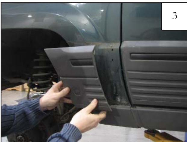
Remove upper factory side cladding piece from front fender.
