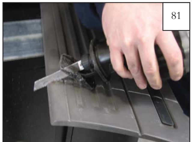
Using a reciprocating saw, cut the body side molding along line drawn in step 78.
