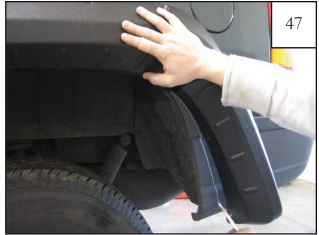
Trace the wheel well edge of bumper flare onto bumper.
