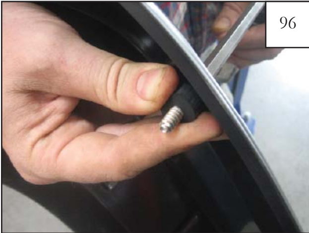
Put screw through hole in pocket of rocker panel piece and secure with rubber grommet using supplied #45 Torx bit. Drive screw into grommet until tight.
