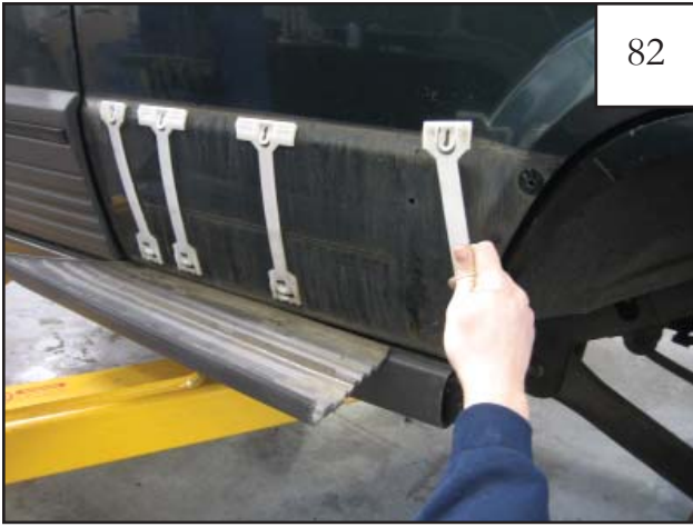
Remove cladding clip closest to the rear wheel well.
