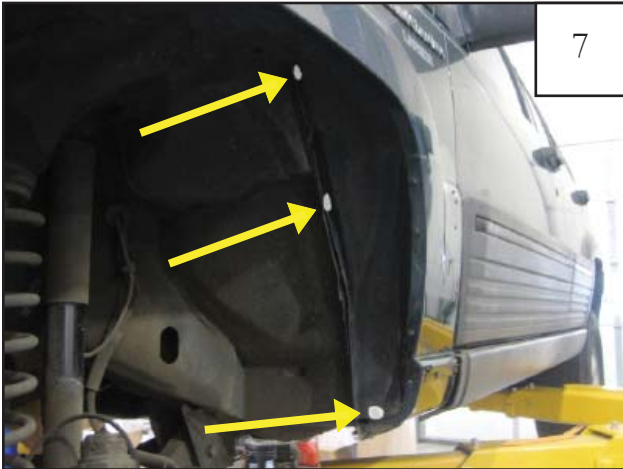
Remove three christmas tree fasteners from wheel well splash shield. Fasteners are white in picture for visibility.
