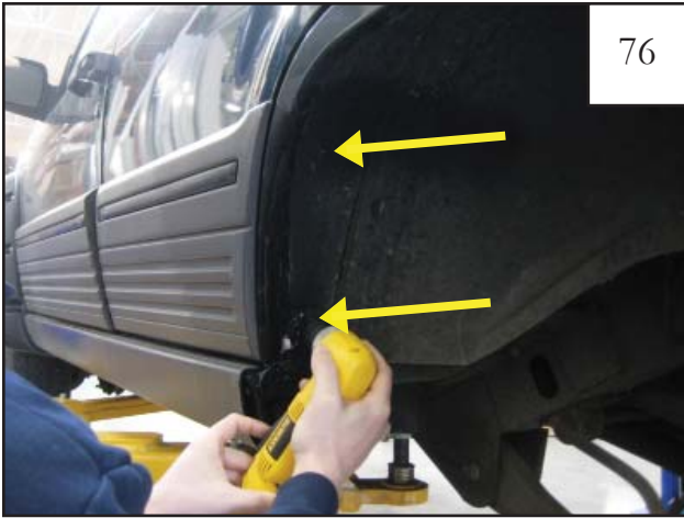
Remove part and drill marked locations with 3/32" drill bit.
