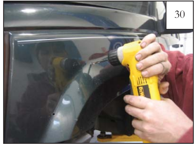
Drill holes in fender at marks made in Step 29 with a 3/16" drill bit.
