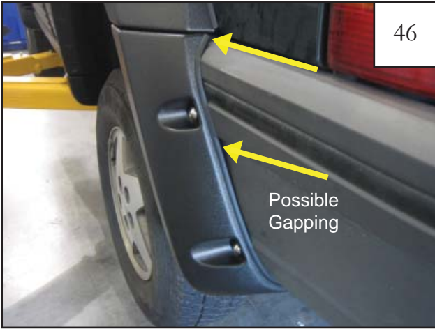
There are three different styles of bumper for this vehicle. The bumper piece may not fit exactly. Gapping may occur. The bumper piece is made to accommodate all three styles.
