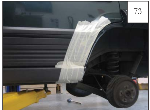
With door open, run masking tape along door edge. Close the door and tape over the side cladding and rocker panel.
