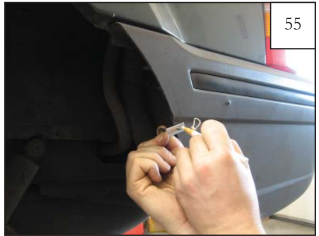
Hold mounting bracket over mark made in Step 54 and make a mark position for hole location. Repeat for second bracket.
