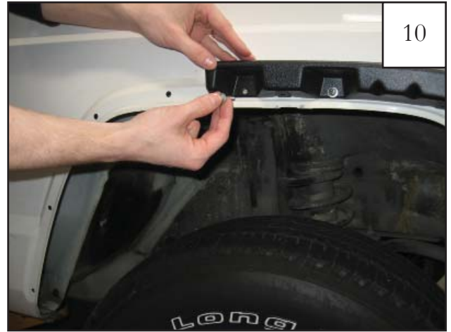
Slide washer onto M5-8 machine screw. Insert a screw/washer assembly through inner flare piece and fender and secure with a flange nut. Only hand tighten at this time.
