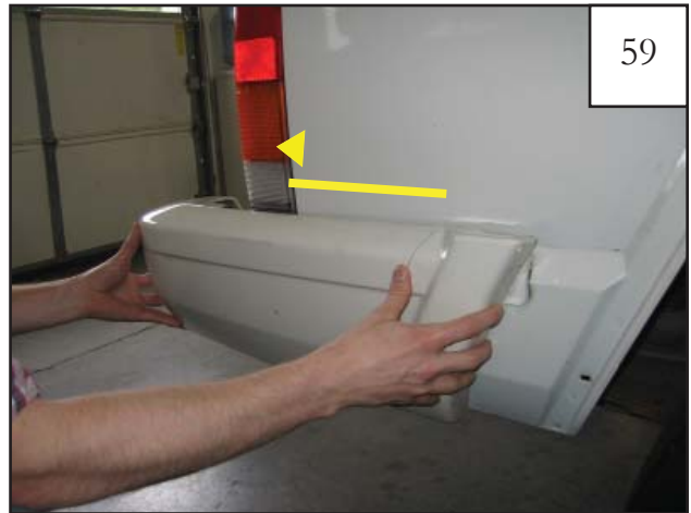
(For 97-01 Model Years Only) Remove the rear factory bumper piece by sliding it toward the rear of the vehicle. Save for optional trimming and reinstallation.
