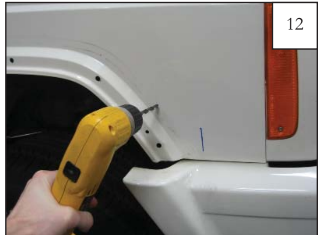
Remove inner piece from front fender. Using a 1/4" drill bit, drill through sheet metal on location marked in previous step. Pre-drill with a smaller drill bit if desired.
