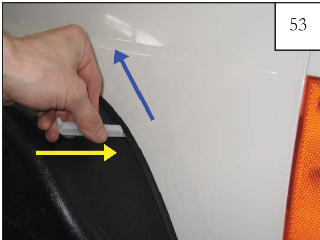
Starting at one end, place the flat edge of the supplied edge trim tool between the lip of the edge trim and the surface of the flare then slide along the edge trim while pressing it in toward the vehicle surface to further ensure proper adhesion.
