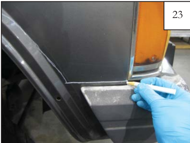
23 (For 84-96 Model Years Only) Use a grease pencil or marker to make a horizontal line extending from bottom of front marker light to profile line made in step 22.
