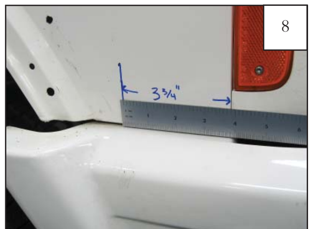
Use a grease pencil or removable marker to mark a vertical line 3-3/4" from the front edge of the sheet metal on the fender.
