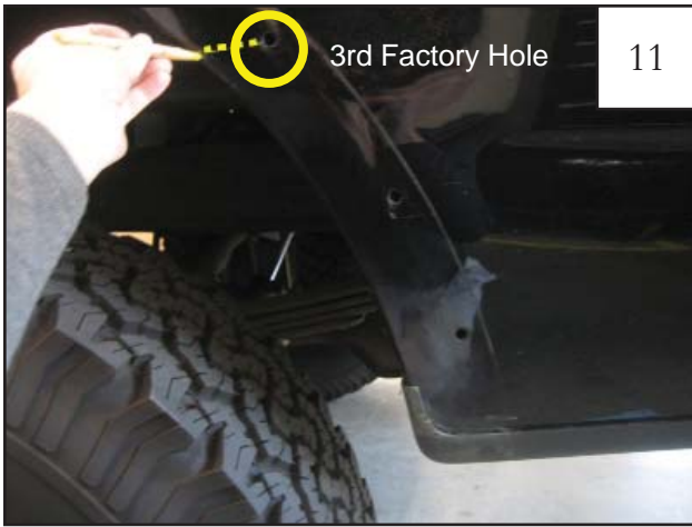
At fender lip, mark a line horizontal to the third factory hole up from bottom front of fender well.
