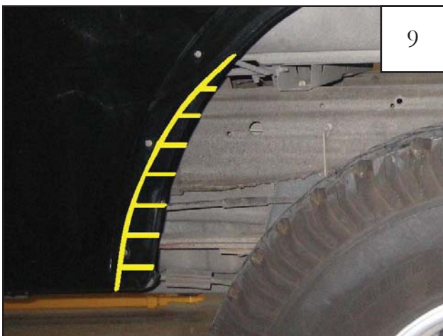
At 1-1/2" intervals, make horizontal lines from fender lip to line drawn in Step 8. These lines will be cut later, forming tabs to be hammered in.
