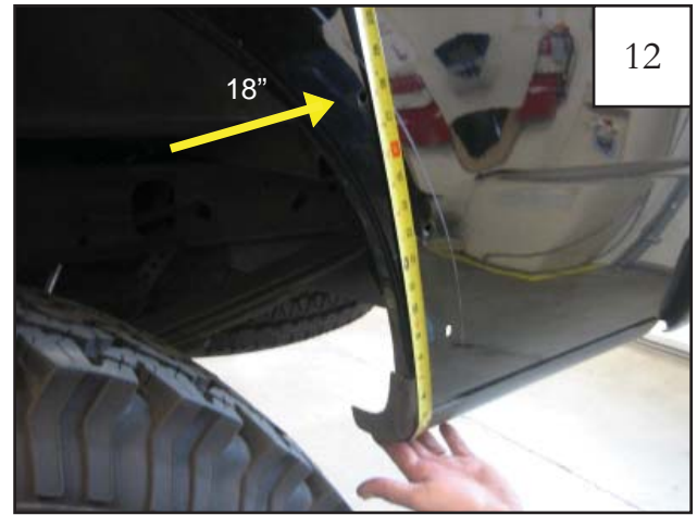
For trucks without factory flares ONLY: Wrapping tape measure up from underside of fender, measure up 18" and make a mark on fender lip where tape measure intersects.
