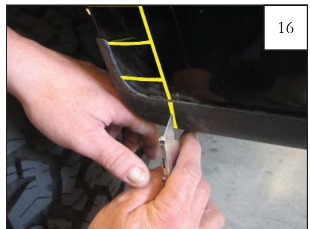
Using a utility knife, cut rock guard along line drawn in Step 15. Peel and discard forward portion of rock guard, leaving rearward portion on the vehicle.
