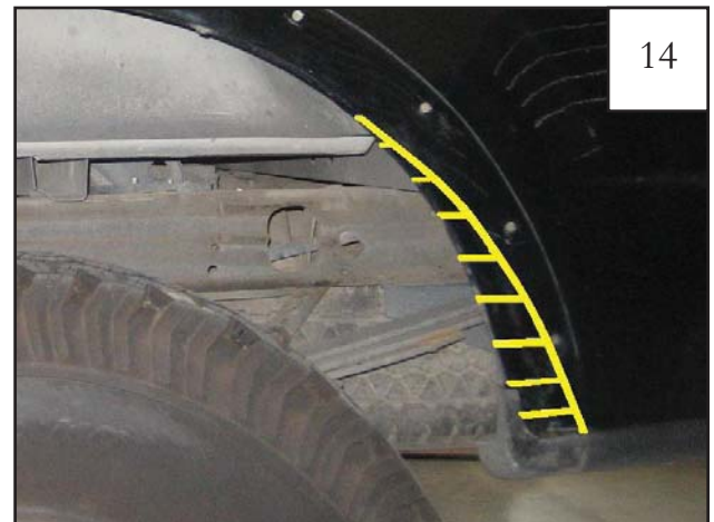
At 1-1/2" intervals, make horizontal lines from fender lip to line drawn in Step 13. These lines will be cut later, forming tabs to be hammered in.
