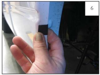
Wrap a Tab (MT1-0014) around the wheel well sheet metal, centered over each of the four marks made in Step 5.
