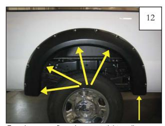
Ensuring proper flare placement, tighten all screws.
