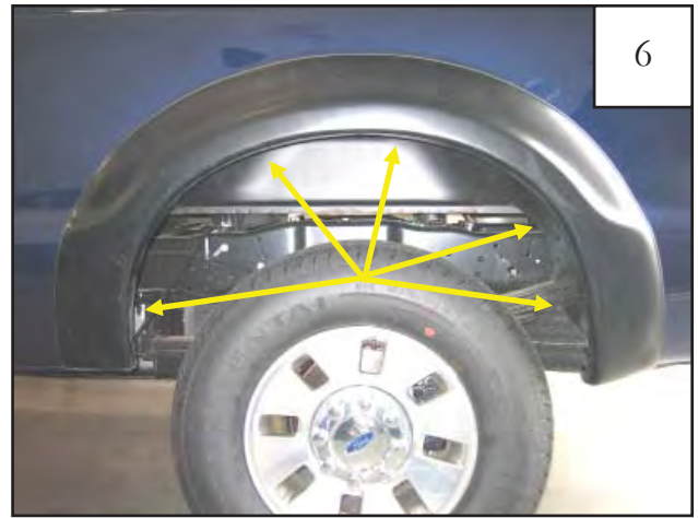
Clip locations. Align these with the holes in the part.
