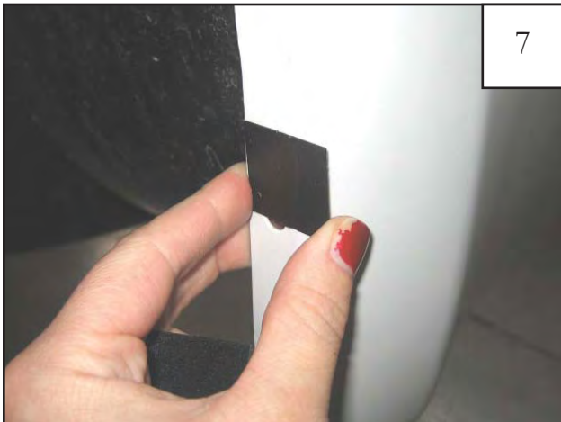
Remove flare and center a black plastic tab over each location marked in Step 5.
