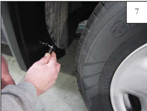
Position and hold flare on fender and reinstall rear most factory screw using a 7/32" socket wrench.
