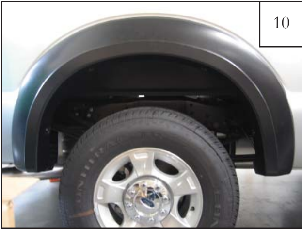
Completed rear flare installation.
