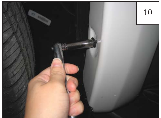
Start three supplied Hex Screws through three rear holes in flare and into factory holes in rear of wheel well.
