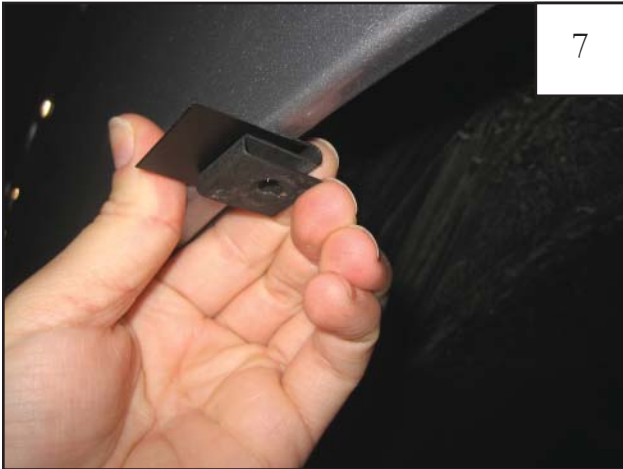
Slide a supplied "S" Clip over each Tab.
