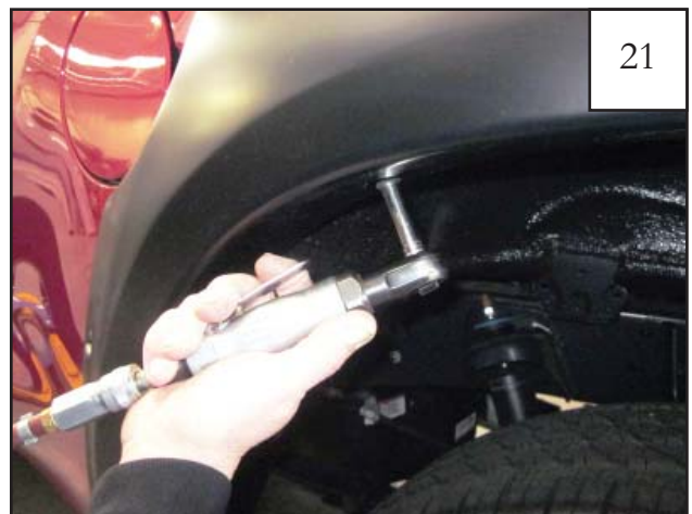
Ensure flare is properly positioned and tighten all screws.
