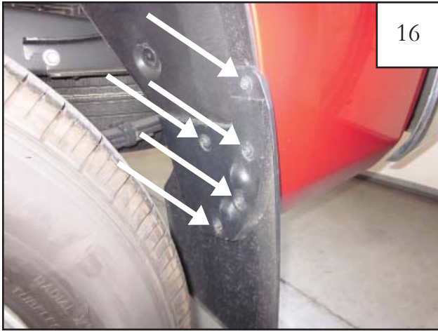
Remove five hex bolts from factory mud flap using a 10mm socket.
