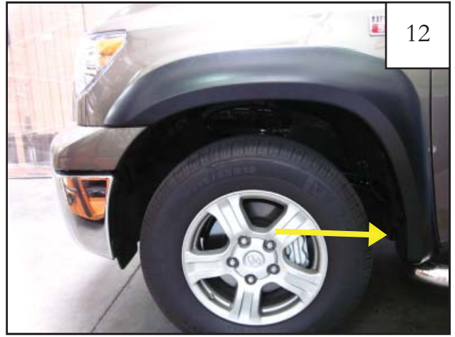
Screw (SW1-0036) lower rear wheel well location.
