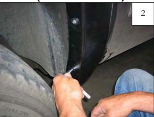
Position flare on fender, and reinstall four factory screws removed in Step 1. If needed, use an awl to locate holes.
