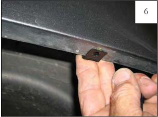
Slide a supplied Plastic Clip over two top factory holes. Clips may need to be adjusted to align with holes in flare. NOTE: the raised collar on the clip should face upward into the interior of the fender.
