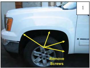
Using a 7mm socket, remove four factory screws. Retain screws for later use.
