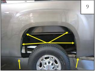
Black Plastic Tab locations. On two underside locations, apply a second tab over the first to increase thickness and prevent clips from falling off.
