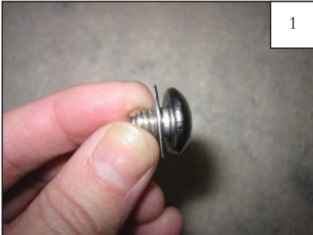
Put a Washer (WA1-0012) on each Bolt (SW1-0059).
