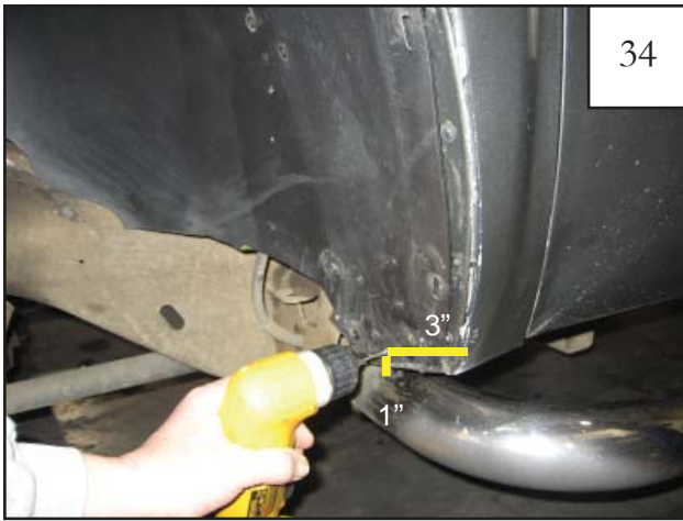
Put splash shield back in place. With a 3/32" bit, drill a hole 3" in from corner of fender and 1" up from bottom edge.
