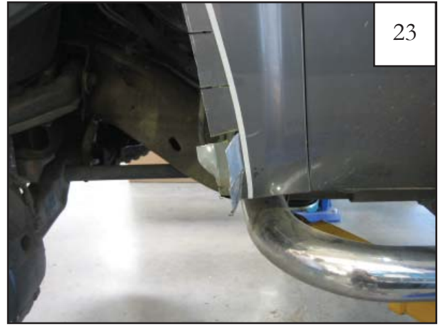
Bend lowest two metal tabs outward.
