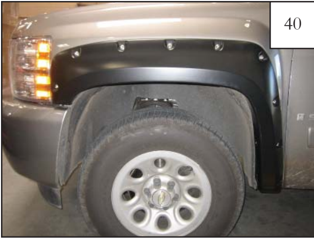
Reinstall wheel. Completed front flare installation.
