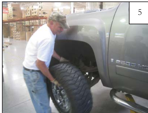
Support vehicle and remove tire.
