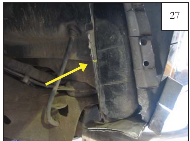
Mark inner pinch seam at location shown.
