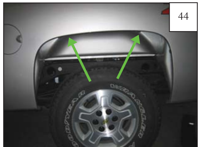
Slide a supplied Clip (CL1-0022) over top two tabs. Clips may need to be adjusted to align with holes in flare.
