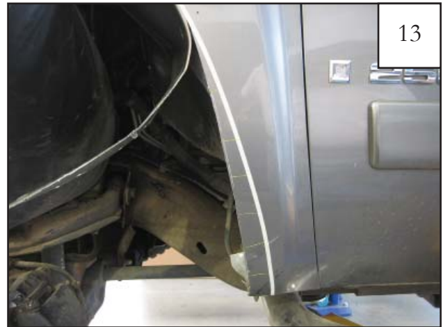
Bend inner fender metal away from fender.
