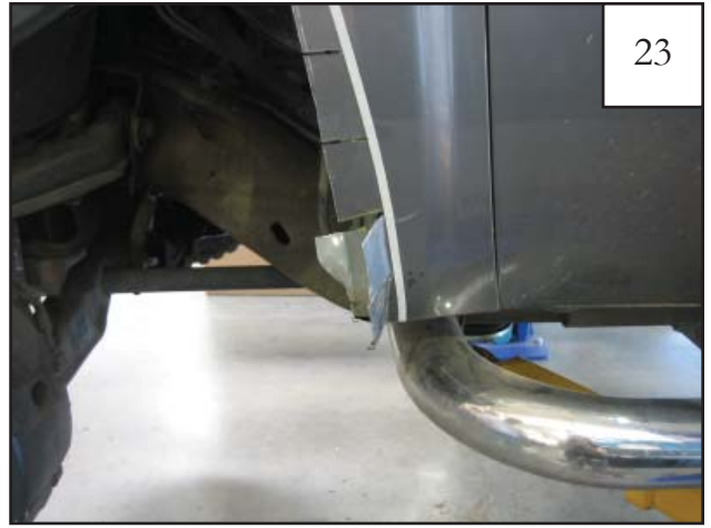
Bend lowest two metal tabs outward.
