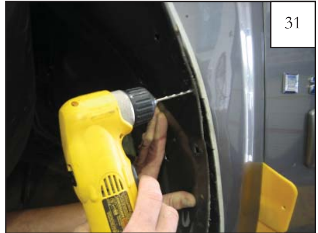
With 3/32" drill bit, drill through mark and the bent tabs of metal behind them for three locations along edge of wheel well.
