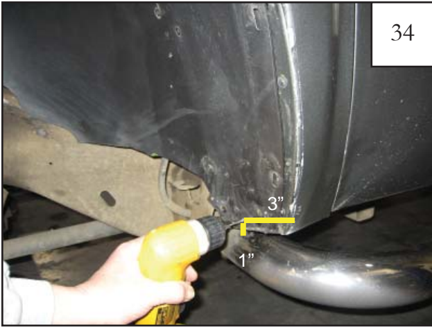
Put splash shield back in place. With a 3/32" bit, drill a hole 3" in from corner of fender and 1" up from bottom edge.
