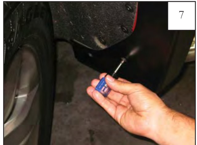
Start supplied Screw (SW1-0056 through two bottom rear holes in flare and into factory hole in rear of wheel well. Do not tighten.
