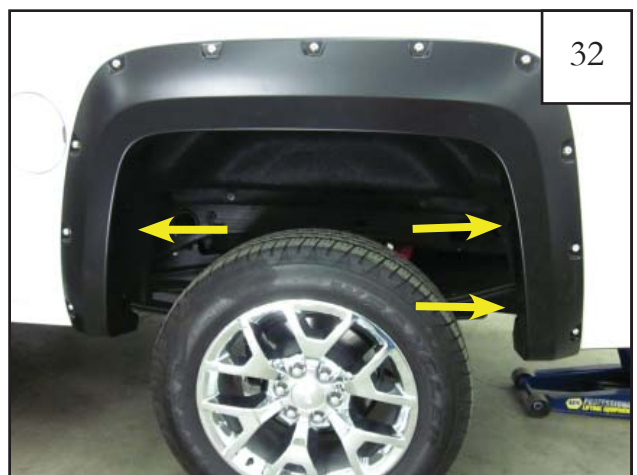
32 Hole locations to be marked for drilling.
