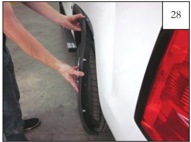
28 Starting at the lower rear end of the factory flare, firmly grip part and pull to remove from vehicle. Note: You will hear popping sounds as the factory fasteners release from vehicle. This is normal.
