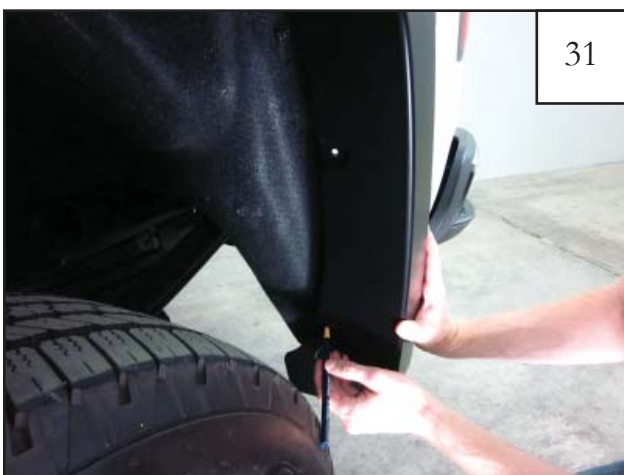
31 Using a grease pencil or marker, hold flare in place on vehicle and mark hole locations for drilling (3 places).
