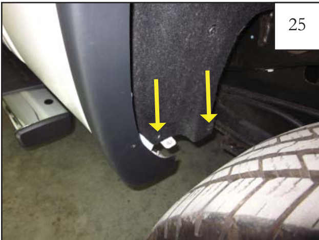
Re-install two factory screws into wheel well liner.
