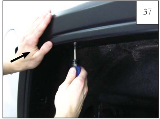
37 Press flare towards vehicle and fully tighten all remaining fasteners.
