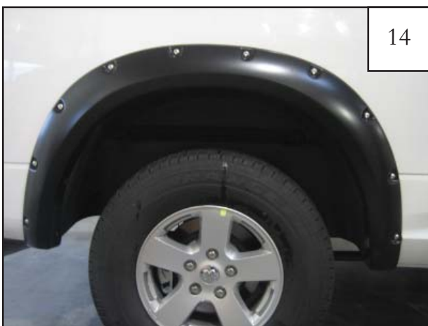
Completed rear flare installation.
