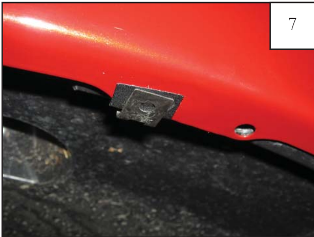
Install speed clip over plastic tab.
