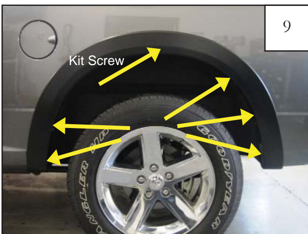
Kit supplied screw and factory installed screw locations. Install the kti supplied screw at the top of flare first for easier installation. See steps 10 & 11.
