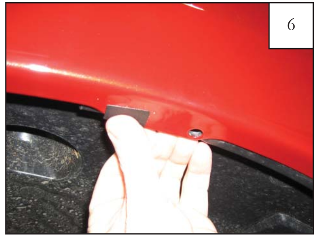
Install plastic tab over existing factory hole.
