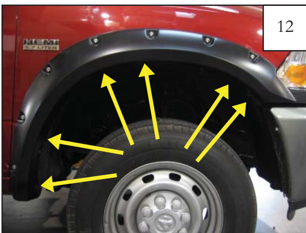
12 Press firmly on flare and tighten all screws.
