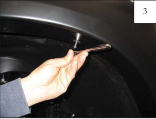
Holding flare in position on fender, reinstall screws removed in Step 2.
