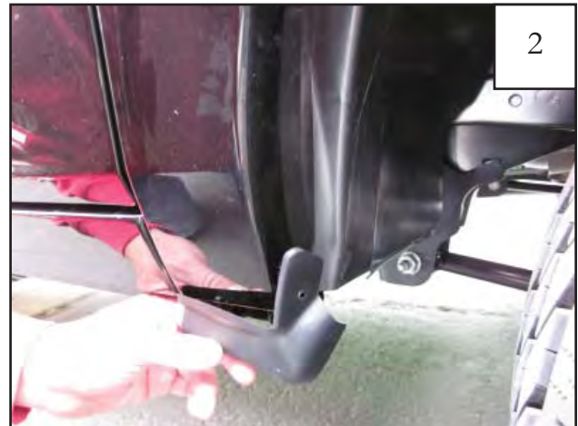
2011 Models Only: Remove inner piece at bottom rear of wheel well.
