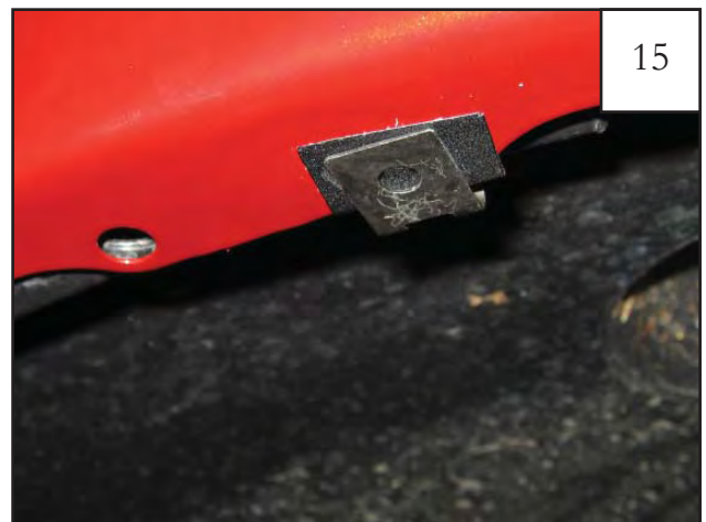
Install #10 U-Clip over 1"x1.5" Black Tab.
