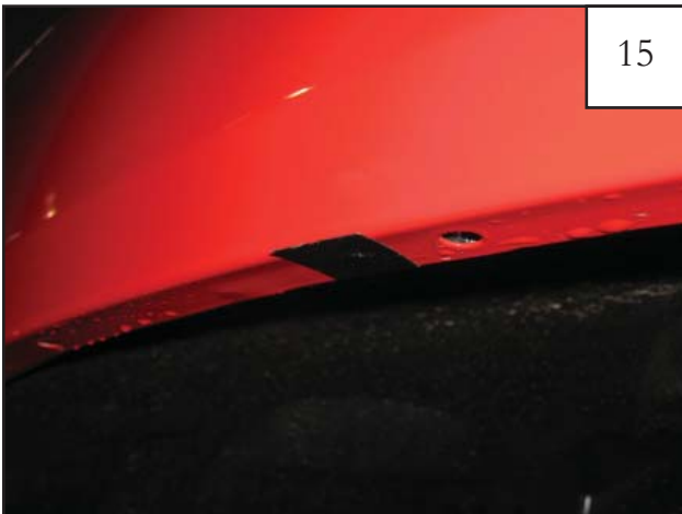
Apply supplied Plastic Tabs along the edge of the fender, centering the tabs on the marks made in Step 4. Tabs should be flush to inner edge.
