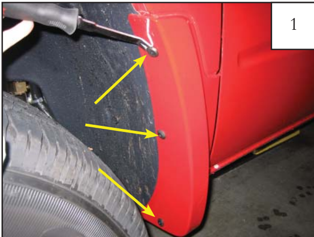
Starting in the rear of the wheel well, remove factory fasteners used to attach mud flap (3 places). Discard fasteners.
