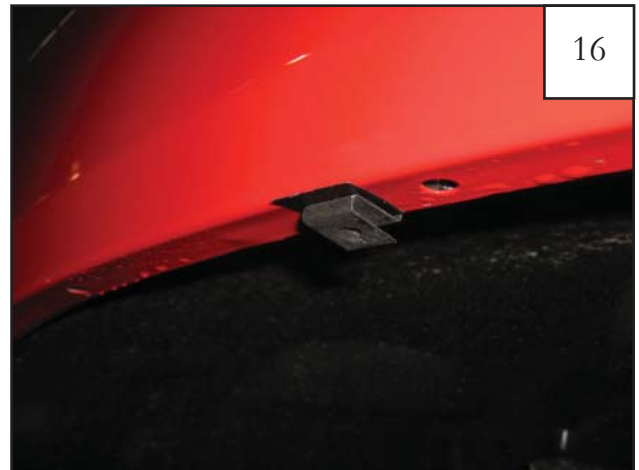
Slide the supplied "S" Clips over the Plastic Tabs on the fender lip (6 places).
