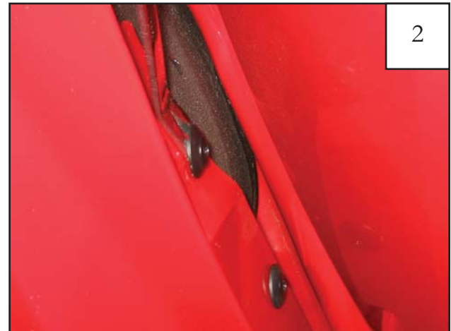
Open door and remove factory fasteners used to attach mud flap (2 places). Discard fasteners and mud flap.
