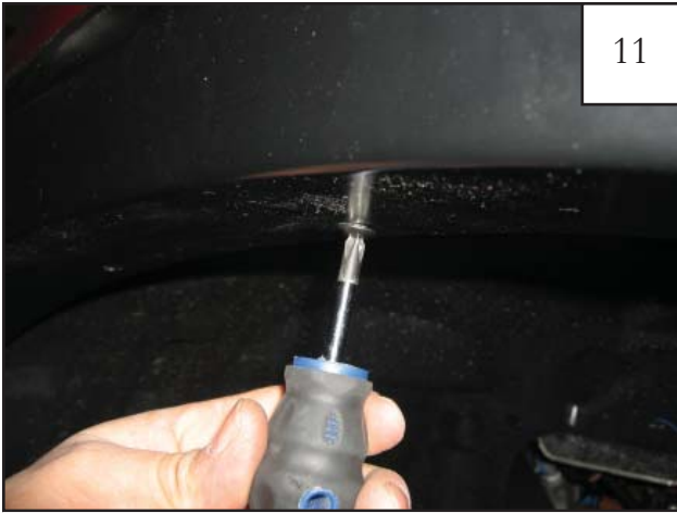
Start supplied Serrated-Flange Screws through the three upper holes in the flare and into the threaded holes in the clips. Tighten all screws.
