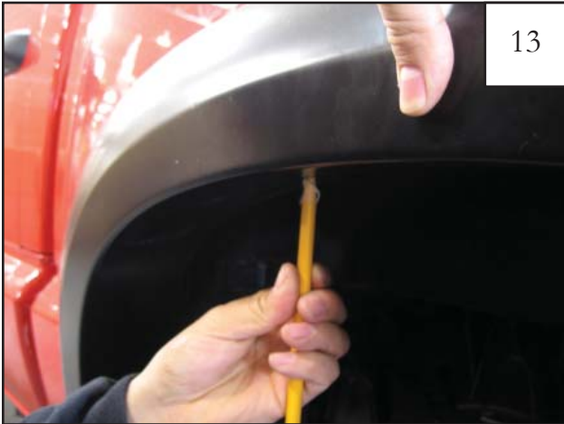
Hold the flare in position on fender. Using the holes in the flare as a guide, mark hole locations on the fender lip with a grease pencil (6 places).
