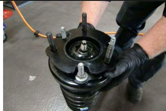
Place upper strut extension on top of coil-over assembly, reinstall and tighten to factory spec using OE hardware.
