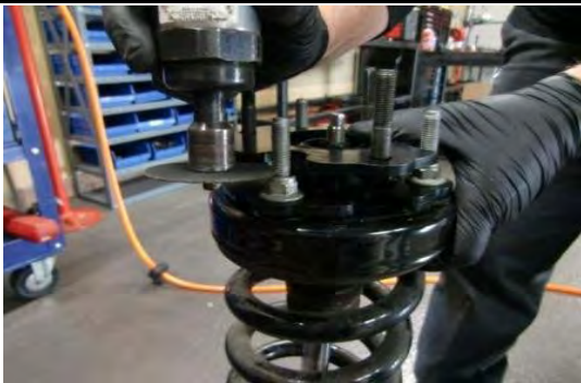
With a cutoff wheel or appropriate tool trim OE mounting studs just under flush with the top of the 66-2055 as shown.
