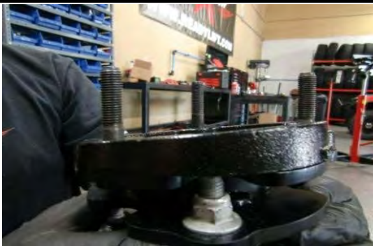
Up close side view of properly installed extension and OE wedge. Reinstall coil-over into vehicle and reassemble in reverse order and tighten to OE specs.
