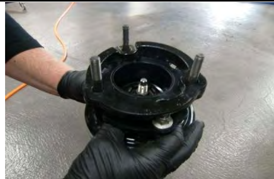
Place wedge on top of the 66-2055 spacer in its original configuration. Note the coil-over will now be installed 180 degrees opposite of the original position.
