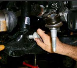
8) Make sure the upper sway bar end link gets reinstalled at this time. Torque to factory specs.
