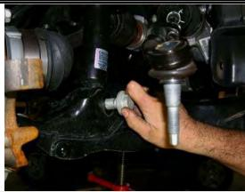
5) Remove the two lower control arm mounting bolts. Use a jack to support the lower control arm and take pressure off the bolts during removal. Below: Remove the three upper strut mounting nuts. Push the lower control arm down a little and remove the strut.
