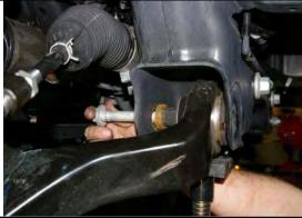
10) Tighten the upper ball joint. Torque to factory specs. Tighten the three upper strut mounting nuts, reinstall the tie rod end, and tighten the lower strut mounting nut. Install the two 10mm brakeline support bolts. Install ABS line back into the brake line support.
