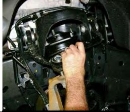
7) Install the lower strut mounting bolt, do not tighten.
