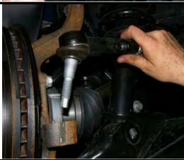
3) Loosen but do not remove the upper ball joint nut. Break the upper ball joint loose from the steering knuckle. DO NOT REMOVE THE UPPER BALL JOINT NUT.
