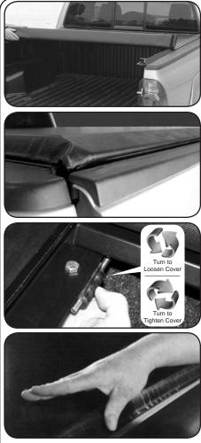
A. Unroll cover and place rear bar into strikes on side rails and press down on bar to close (20-30 pounds pressure).
