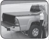
Now along side of box, seal cover edges with hook and loop sealing system the full length of cover on both sides. Pull with one hand seal with other hand.
