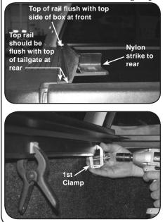
A. Align weatherstrip edge of side rail against inside lip of box **and push forward until it stops against front of box** (nylon strike goes to rear). At front, rail should be flush with top side of box. At rear, rail should be flush with top of tailgate.
