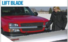
To begin plowing, remove pin, lift blade one end at a time and lower it over push frame, then replace the pin.
