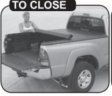
Release retainer straps at front and using both hands roll cover out to rear of box.
