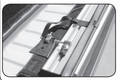
B. Turn 1-1/4" bolt with flat washer onto nut in bar. Leave loose for now. See photo. Repeat for XT-Dial ("R") on passenger side of cover, and leave that bolt loose also.
