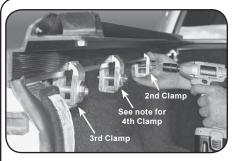
C. Install 2nd clamp on rail at midway point of box. Check if rail is level. If rail tilts up, loosen clamp, lower it and tighten. If rail tilts down, loosen clamp, raise it and tighten. Install third clamp as close to tailgate as possible.
