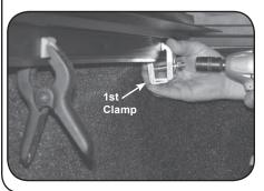
B. Hold rail in proper position with spring clamp. Install 1st clamp as close to front as possible and use ½" wrench to tighten.
