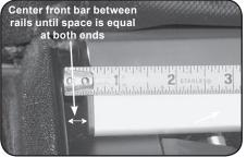
D. Center the front bar between the two side rails.
