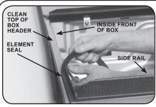
A. At front of box header, clean top surface with alcohol pad (if needed wash first).
