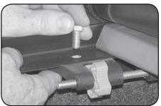
B. Slide left tension adjuster over until it engages under side rail. Push bar back and forth to line up holes—do not turn dial wheel. Insert bolt from top and flat washer and nut from bottom.
