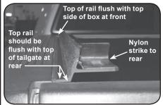
A. Position side rail with weather strip against inside lip of box. **Push forward until it touches front of box** (end of rail with strike goes to rear). At front, rail should be flush with top side of box. At rear, rail should be flush with top of tailgate.
