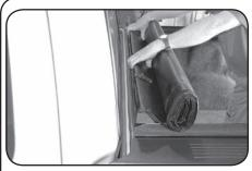
A. Set rolled up cover on rails at front of box (behind cab) with bar facing up. Roll cover bar onto front of rails and fold/tuck vinyl flap under. Now bar will face down. Let straps hang to inside of box. Push cover bar forward until it sets flat on front of side rails and overhangs them.
