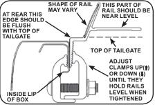
D. When done, make sure each clamp is in its best up or down position to hold rail level after tightening and that all clamps are fully tight. Repeat entire procedure for opposite side rail.
