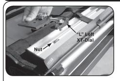
A. The cover comes pre-rolled to its normal open position for ease of installation. Set pre-rolled cover on tailgate with front bar facing up as shown. Align XT-Dial Tension Adjuster (marked "L") on driver side of cover—positioned as shown in photo.
