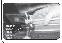
E. Then tighten bolt (left loose earlier) under front bar on each tension adjuster.
