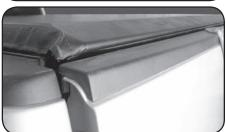
B. Close tailgate slowly—top of tailgate should fit snug under cover bar. If it is too tight—raise rails by loosening rear clamps, adjust rail up and tighten clamps. If too loose, adjust rails lower.
