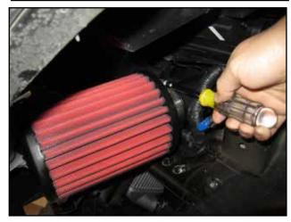
e. From the driver's side wheel well, install filter(E) onto lower pipe and secure with provided hose clamp(F).
