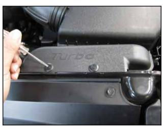
d. Remove the two plastic clips shown above and pull up on the air inlet snorkel to remove.
