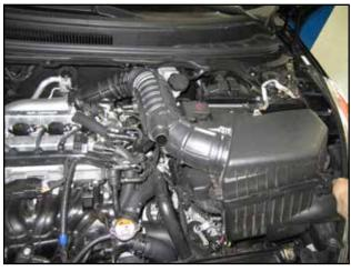
f. Firmly grasp the airbox and slide it towards the engine to detach from lower chamber. Remove stock intake airbox and tube assembly.
