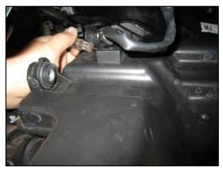
I. Carefully lower the intake resonator and disconnect the tree mount clip to detach the foglight harness. Set aside resonator chamber.
