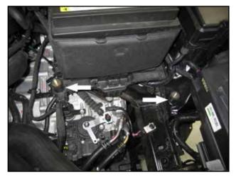
Install the two rubber mounts(I)
