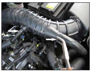
b. Loosen spring clamps to detach crank case breather hose and recirculating valve hose from intake tube.
