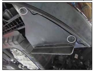
Remove the two plastic clips under vehicle, near driver's side front wheel to lower plastic wheel well liner.
