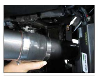
d. Slide provided coupler(B) over non-stamped end of lower pipe(D) along with two hose clamps(C). Slide stamped end of tube down below driver side headlight housing and position mounting bracket into second rubber mount. Slide coupler evenly between upper and lower tubes. Ensure proper clearance between tube and headlight housing.
