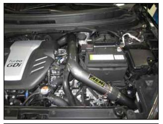
AEM cold air intake system installed.
