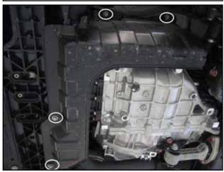
Remove four silver M6 bolts securing lower plastic belly pan cover.
