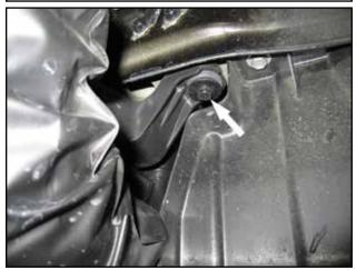
From driver's side wheel well, remove the M6 bolt used to secure the intake resonator chamber rear mount.
