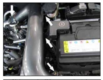
c. Slide coupler(B) over turbo inlet with two hose clamps(C). Insert tube(A) into coupler and position bracket into rubber mount as shown, leaving clearance between tube and brake fluid reservoir and positive battery terminal.
