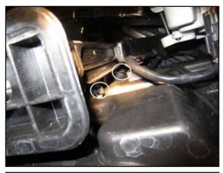
k. From underneath vehicle, remove the remaining two M6 bolts securing the lower intake resonator.
