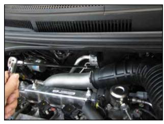
Loosen the stock hose clamp on turbo inlet using a 10mm socket and ratchet.
