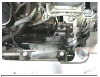
a. Install the scoop back into the vehicle and secure with the bolts that were removed in step 2c.
