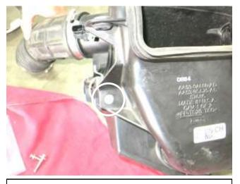
f. Remove the bolt that secures the air scoop to the lower air box. The bolt will not be reused.
