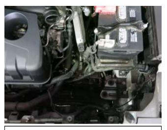
d. Remove the complete air intake assembly from the vehicle. NOTE: DO NOT DISCARD ANY OF YOUR STOCK EQUIPEMNT.
