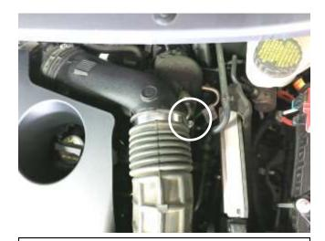
b. Loosen the hose clamp at the turbo inlet pipe.
