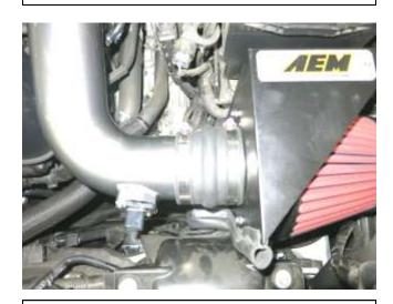
j. Slide the AEM intake tube into the coupler. Do not tighten the hose clamp at this time.
