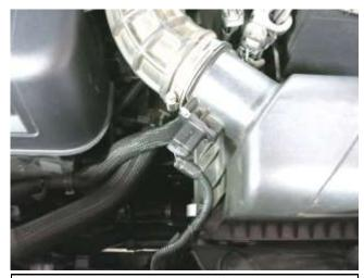
a. Slide the red locking tab and detach the electrical connector from the sensor.
