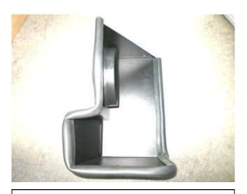
d. Install the provided edge trim onto the heat shield, cutting to fit as shown.
