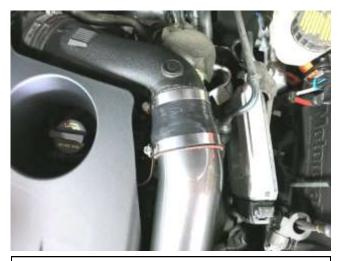
k. Slide the other end into the previously installed coupler on the inlet tube. Secure both hose clamps now once proper tube alignment has been achieved.
