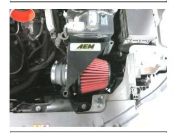
i. Install the complete heat shield assembly into the vehicle sliding the lower portion of the heat shield under the scoop and aligning the plastic mounts in the grommets.
