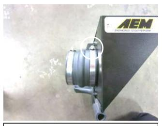
f. Install the provided coupler onto the heat shield air filter adapter. Tighten the hose clamp closest to the heat shield at this time.
