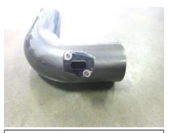
b. Install the sensor that was removed in step 2e and secure in the AEM intake tube with the provided hardware.
