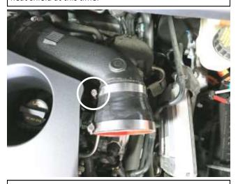
h. Slide the hose onto the turbo inlet pipe with the hose clamps and tighten the one closest to the pipe.
