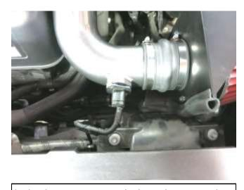
I. Plug the sensor connector back into the sensor and slide the red locking tab in that was removed in step 2a.
