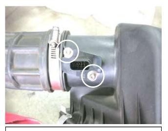
e. Remove the two sensor screws and the sensor. The sensor will be reused in step 3b.
