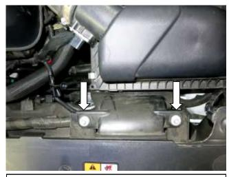
c. Remove the two bolts securing the air scoop to the vehicle. The scoop will be reinstalled in step 3a.
