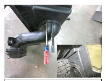
g. Unclip the latches to separate the upper and lower air box. Insert two small flat head screwdrivers as shown into the scoop and lightly put pressure to release the clip securing the scoop to the lower air box. NOTE: The picture in the lower right hand corner shows the screwdrivers inserted on both side of the clip.
