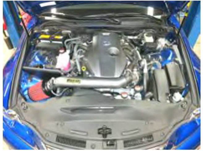
AEM INTAKE INSTALLED
