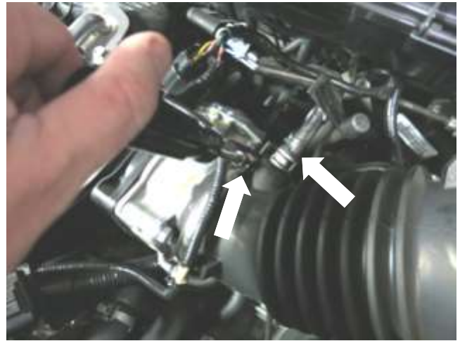
f. Loosen hose clamp at throttle body side of intake hose and remove the vent tube by releasing the pressure on the spring clamp while pulling the vent tube.
