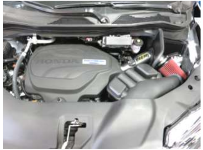
AEM INTAKE INSTALLED
