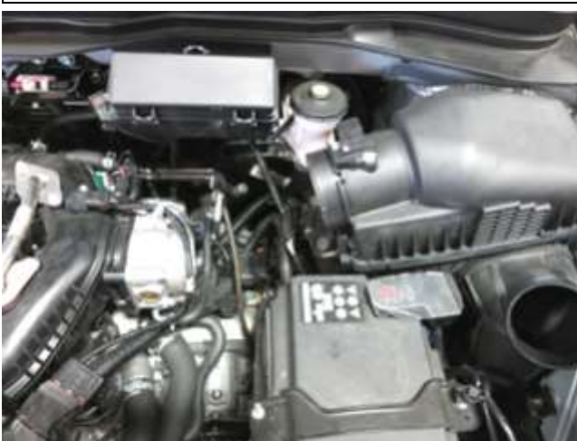
i. Remove the stock intake hose by first removing it from the air box and then collapsing the bellows so it can clear the air box. Then, remove it from the throttle body and engine bay.
