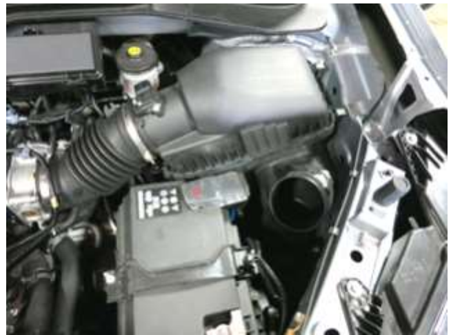
h. Lift out cold air scoop, leaving rubber coupler on cold air scoop.
