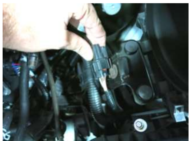
j. Unclip the three wire harnesses from the air box bracket by depressing each latch and sliding them from the clips.
