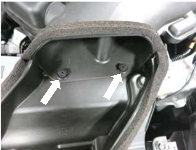
g. Remove the two plastic pop-out mounts securing the cold air scoop by unscrewing them with a Philips screw driver. Note: Use care to not drop the clips as they are easily lost in the core support area.
