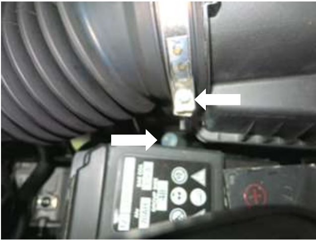
e. Unbolt the factory air box behind the battery using a long extension and loosen hose clamp at air box side of intake hose.
